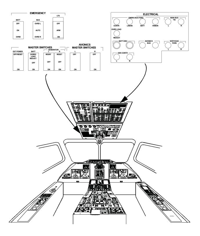
Figure 5-3. Electrical System Controls
