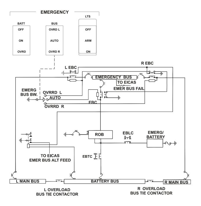
Figure 5-2. Emergency Power System-Schematic
