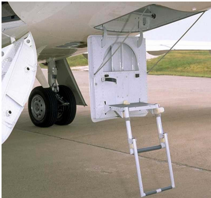
FIGURE 02-50-10-21 MECHANIC SERVICING DOOR
