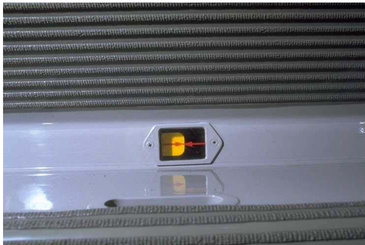
FIGURE 02-50-10-12 VISUAL INSPECTION WINDOW
