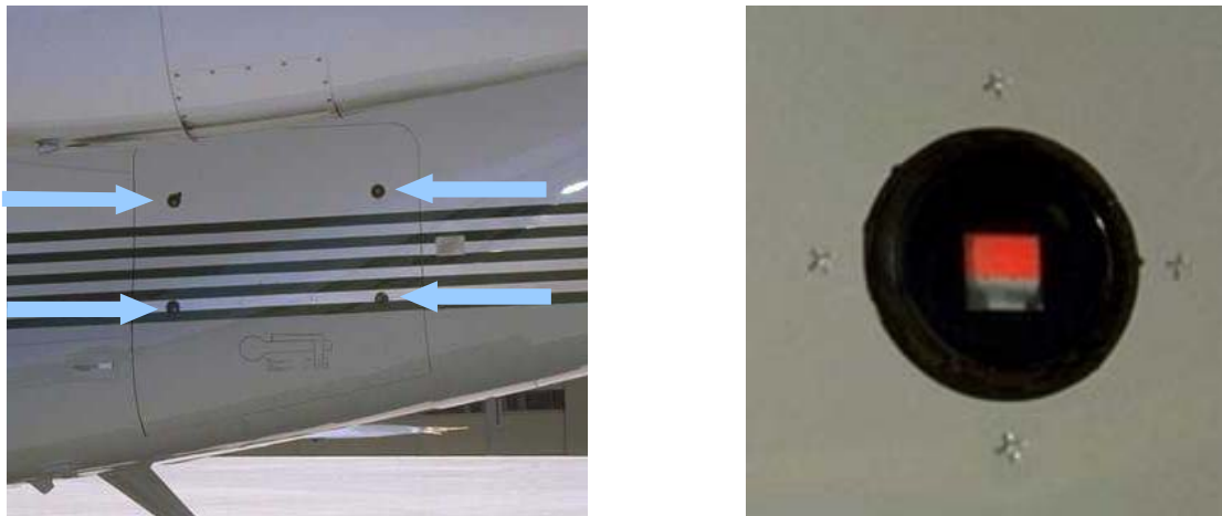
FIGURE 02-50-10-20 RED MARK AND VISUAL INSPECTION WINDOWS
