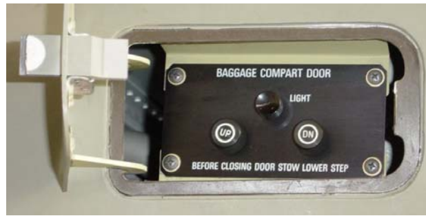
FIGURE 02-50-10-19 CONTROL ACCESS PANEL
